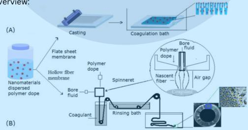
The phase inversion process typically starts with the dissolution of a polymer in a suitable solvent to create a homogeneous solution. This solution comprises the polymer in a dissolved state, along with additives or modifiers aimed at achieving specific membrane properties.
